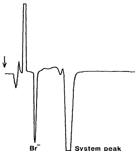
Fig. 7. Sample dissolved in water. Mobile phase: 3 \cdot 10^{-4} M 1-phenethyl-2-picolinium in 0.1 M acetic acid. Solid phase: \mu Bondapak Phenyl. Sample: bromide.
